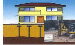
Ground reinforcement method using wooden piles
