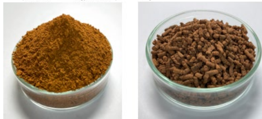
*1 Solid sorbents for CO 2 capture Industrial production using Toda Kogyo's proprietary iron oxide synthesis technology
